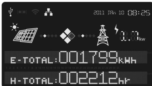
1. E-Total & H-Total: E-Total (total accumulated energy) in kWh and H-Total (total operating time of inverter) in hours
